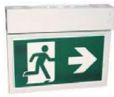
EB81010033 Wall,Ceiling Standby:1-3 Hours 330*248*45mm 30 meter Viewing
